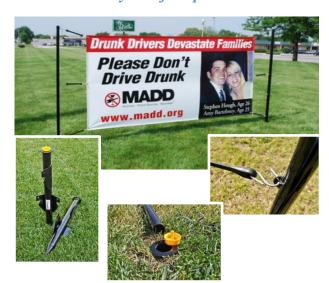
There are (2) pole sleeves that are installed into the ground and (2) poles that can slide in and out of the sleeves. The poles are 7' long and install 22" into the ground sleeves. The banners are suspended from the poles using rubber bungee straps. The entire system is powder coated for rust resistance and an attractive finish.
